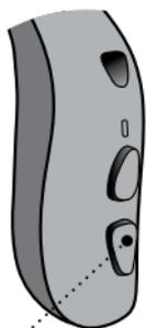
To activate and deactivate flight mode press and hold the push button (lower part) for 7 seconds.
