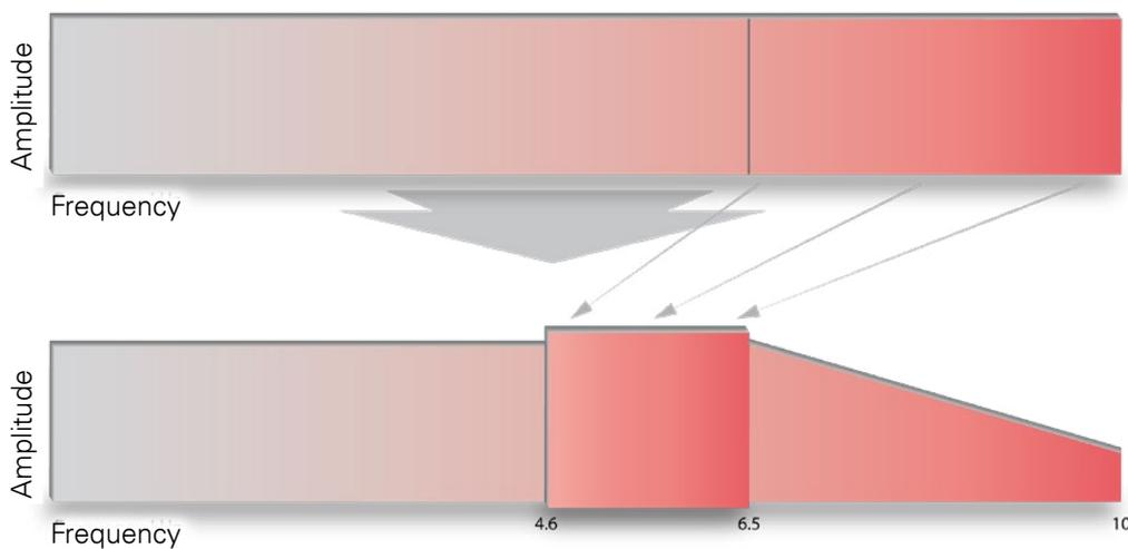
High-frequency information is transferred and superimposed to a lower frequency destination. The entire original signal can be amplified or the high frequencies can be attenuated.
