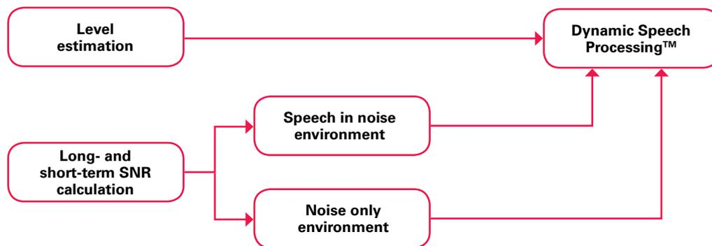
Working simultaneously with the level estimation, DAC™ calculates the long-term and short-term SNR as well as determines the presence of speech in the environment and then transfers this information to the DSP™.
