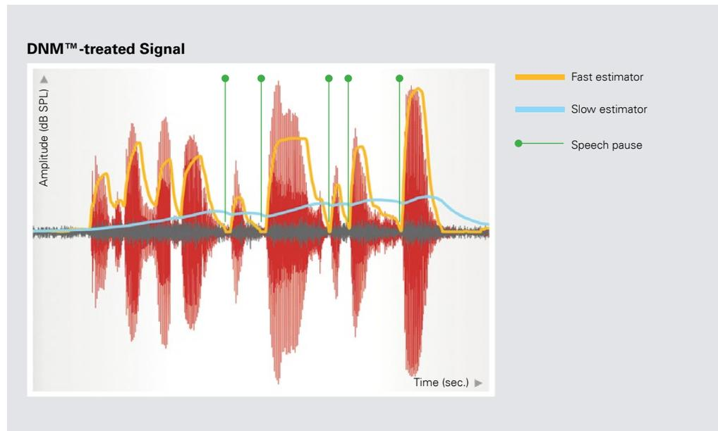
A speech signal (red) with background noise (gray), showing the long-term and short-term SNR measurements. The noise within the highlighted speech pauses could potentially be amplified; however, by using the information provided by both SNR measurements, the DSP™ applies an optimized amount of gain and compression to avoid over amplification of noise.
