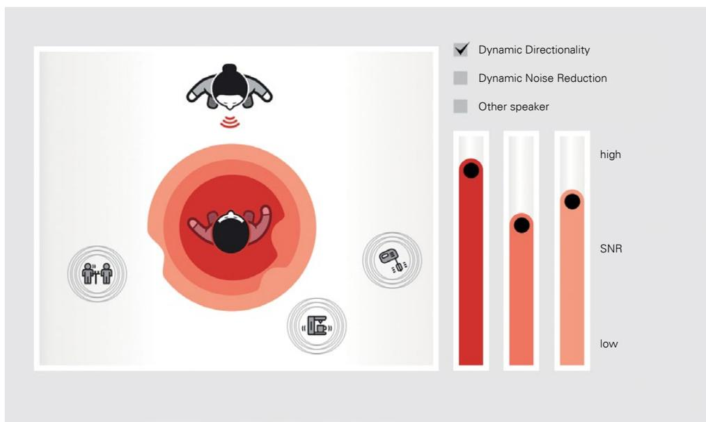
Dynamic Directionality alone (top) may be enough to achieve the best possible SNR. The multiple directionality patterns set their null points to reduce noise from various angles. When noise from another angle is added (bottom), the Dynamic Noise Reduction will activate and reduce the additional noise source.
