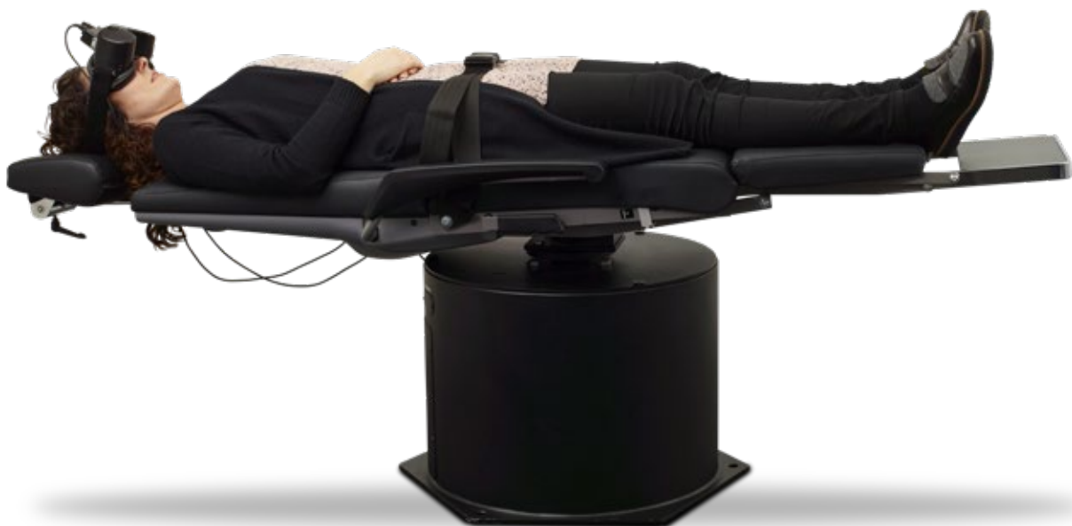
To assure a correct angle for caloric testing, an indicator resides on the side of the chair.
