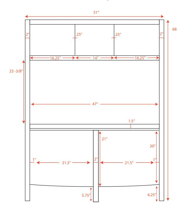
Depth of counter: 12.25" - 16.25" curve Backplate: 46.75" w x 23.5" h HIT shelf: 15" w x 14" d HIT open: 12.5" h Camera shelf depth: 6.5" - 7" curve Side of unit: Black beam is 5" deep Hat track: 7.5" h REM approx: 14.5" x 17" Arms extend out to side: max 26"
