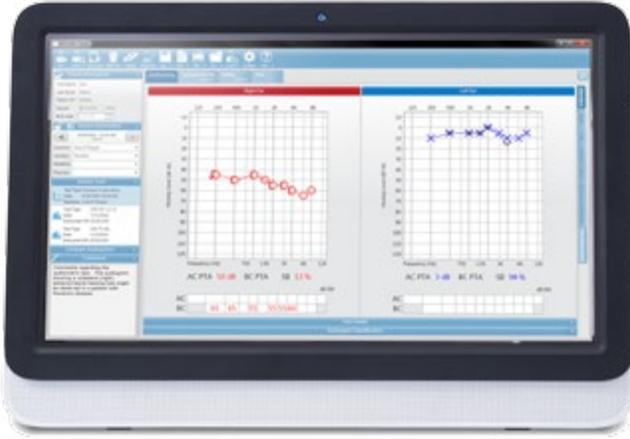
With a single button press, data is transferred from a GSI instrument to GSI Suite™, where it is stored and custom reports may be generated. Audiometric, tympanometric, and OAE test results can be combined into predefined or fully customized report templates. Additional features include counseling overlays for immediate feedback to the patient and Noah compatibility.
