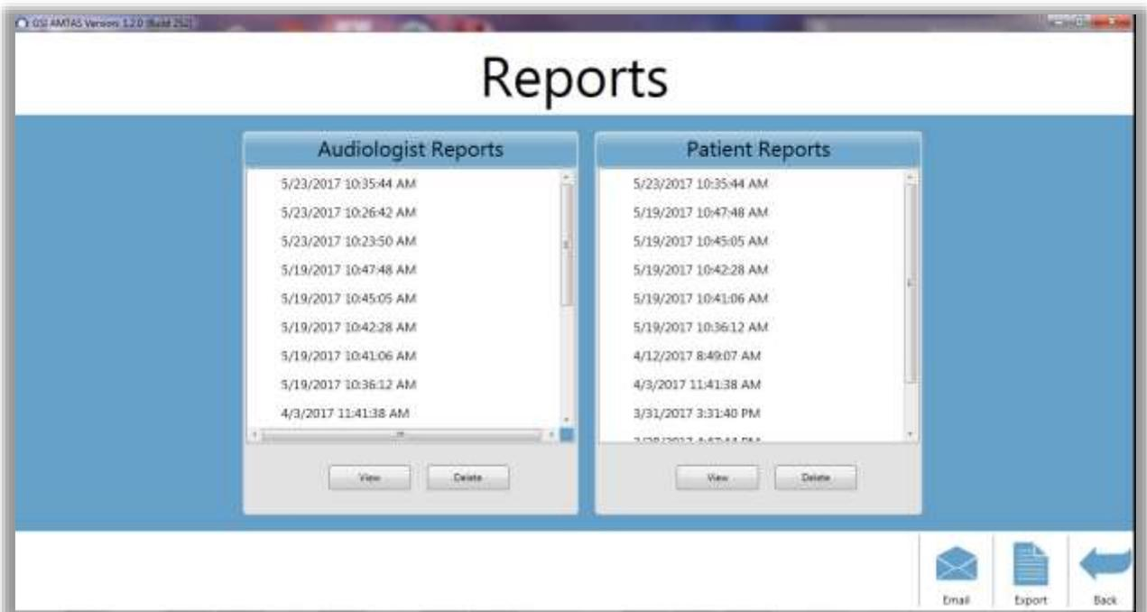
The menu bar at the bottom of the screen has buttons that are used to send the report to an email address or to export the report to another location. Sending a report by email requires that an email client is installed on the PC. When the Email button is selected, the default email client displays its send dialog where you enter
