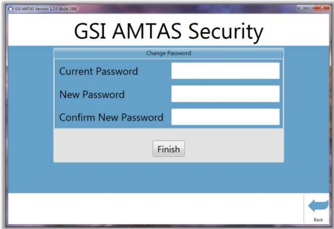
To change the password you must enter the old password, then enter the new password and a confirmation of the new password. Press the finish button to save the new password, then the Back button to return to the main screen.
