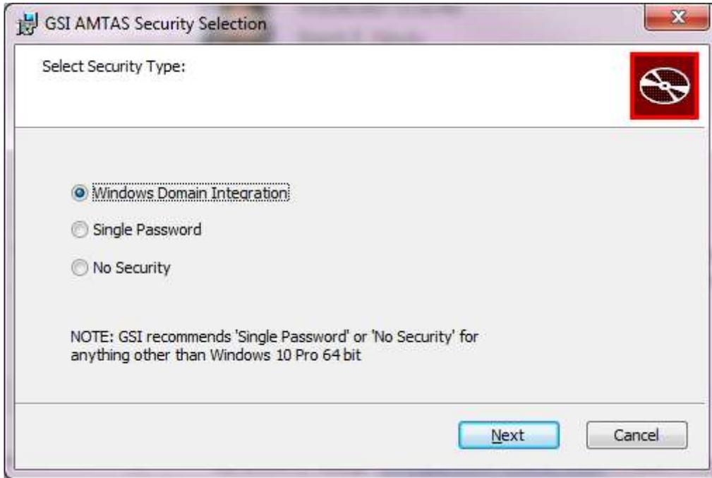
4. The type of security that is used with the program is setup during the installation. A security selection dialog is presented with three (3) security options. Select the appropriate security type for your facility.
