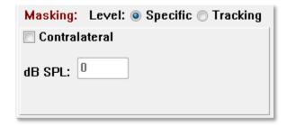
The Masking Level may be specified in two different ways. The Specific level provides the masking at the fixed level specified in the dB SPL field regardless of the stimulus level. The Tracking level delivers the masking noise at a level relative to the stimulus level. When the Tracking level is selected, the dB SPL field represents the offset relative to the stimulus. For example, -20 would indicate that the masking would be presented at 20 dB less than the
