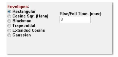
The Rectangle, Cosign Sqr. (Hann), Blackman, Gaussian envelopes do not have a user specified field for the rise/fall parameter. These envelopes have a 0 plateau, and the rise and fall are each equal to half of the specified duration. The Gaussian envelope is specified in cycles for duration and should be in increments of 0.5 to ensure a smooth transition.
