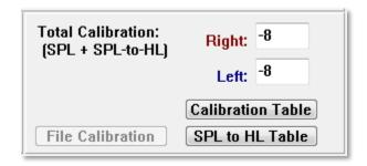
The File Calibration, Calibration Table and SPL to HL Table buttons display the values used in the overall total calibration.
