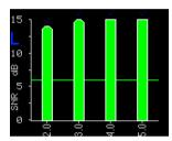
In SNR Mode, when both ears have been tested, press the DOWN arrow key and the results of the last test performed will display. An R or L in the upper left side of the screen indicates the ear tested. Red and blue check marks above green bars
