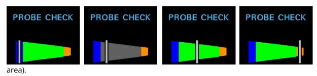
The vertical white bar indicates the measured ear canal volume and probe fit stability:
