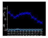
The Value graph view for left ear test displays dark blue "x" symbols representing the absolute emission levels at each DP test frequency or TE frequency band. Light blue upside-down triangles represent the noise floor at each DP test frequency or TE frequency band. For screening protocols, a blue check mark above the blue "x" indicates a pass for that frequency.
