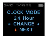
The Clock Mode menu allows the user to change the clock from a 24 hour mode to a 12 hour mode. To change the clock mode, press the ←CHANGE→ keys. Press the ↓NEXT to exit this menu. When 12 hour mode is selected, AM or PM will appear in the time/date screen.
