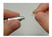
A probe tube must be applied to the probe head before an eartip is applied. Insert a new probe tube into the probe head until it is fully seated. A properly inserted probe tube will snap securely into place when it is fully seated in the probe head. It is not necessary to replace the probe tube with each ear tip; the tube is reusable as long as the probe
