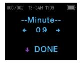
Continue through each menu item until the correct date and time are set. Press the ↓DONE arrow key will return to the Main Menu. The time and date changes are automatically saved.
