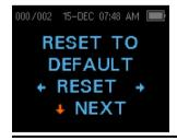
The Reset to Default menu will return all instrument settings and protocol settings to their original factory defaults. Select the  $\leftarrow$ LEFT or RIGHT $\rightarrow$  arrow key to reset and select  $\leftarrow$ Yes or No $\rightarrow$  to verify reset. To exit the System menu without resetting the instrument, press  $\lor$ NEXT to return to the Main Menu.
