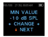
The Minimum Amplitude setting allows the user to set the unit to include minimum amplitude values in the pass/refer criterion. If the MIN VALUE is set to a specific dB SPL value, a result is not considered a Pass unless the amplitude at each frequency is equal to or greater than the minimum value programmed into the unit. This is in addition to meeting the other pass criteria
