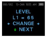
The intensity of the primary tones (L1, L2) may be changed to any level between 40 dB SPL and 70 dB SPL. The level L1 will change in 1 dB increments by pushing the  $\leftarrow$ LEFT or RIGHT $\rightarrow$  arrow keys and press  $\lor$ NEXT to move to the L2 screen.
