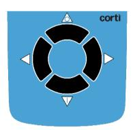
The Corti instrument uses 4 buttons to control all functions of the instrument. These buttons are arranged in a directional cursor format. The arrows on the keypad ( $\leftarrow$ LEFT,  $\rightarrow$ RIGHT,  $\uparrow$ UP, and  $\downarrow$ DOWN) correspond to the arrows that are used on the screen. The screen will indicate which button to push by showing the appropriate arrow.
