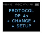
The currently selected protocol is shown on the Main Menu. To change the selected protocol press  $\Psi$ CHANGE at the Main Menu. The Change Protocol display will appear. Use the  $\leftarrow$ CHANGE $\rightarrow$  arrow buttons to change the selected protocol. Press the up arrow to return to the Main Menu to begin testing. Press the  $\Psi$ SETUP to enter the setup menus.
