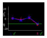
The Corti will display the both Right and Left results at the end of the test, when in Save L/R Mode. After both ears have been tested, press the DOWN arrow key. When in Value Graph, both right and left results will display on the same graph. A green check mark below the graph indicates a pass. An orange 'X' indicates a refer and a '?' indicates Noisy, No Seal, or Fit Err. Red
