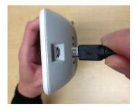
The Corti instrument is powered by an integrated rechargeable lithium-ion battery providing 20hours of operation between full charging. The battery status is indicated by the battery icon shown in the upper right corner of the Main Menu. Full battery charge is represented by a full battery symbol on the display and reduces to an empty battery in increments corresponding to the discharge
