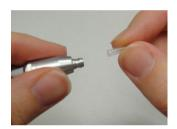
A probe tube must be applied to the probe head before an eartip is applied. Insert a new probe tube into the probe head until it is fully seated. A properly inserted probe tube will snap securely into place when it is fully seated in the probe head. It is not necessary to replace the probe tube with each ear tip; the tube is reusable as long as the probe
