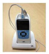
Make sure the probe holder is towards the end of the probe cable at the GSI wave logo / HDMI connector end. Gently push the probe cable into the probe holder at the point of the probe head.
