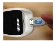
Insert the Probe's HDMI connector firmly into the socket on the top of the Corti. The plug will fit in only one direction. The GSI wave logo will align with the instrument control panel.
