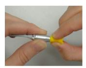
Probe tubes are disposable and should be replaced when they become clogged. Replacement probe tubes are included with this instrument. Do not attempt to clean the probe tube.
