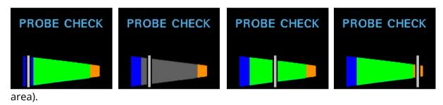
The vertical white bar indicates the measured ear canal volume and probe fit stability:
