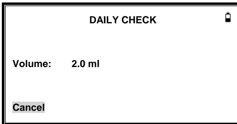
Remove the probe and repeat the test with the three remaining test cavities. The display should show the volume of the 0.2ml, & 0.5ml test cavities to within  $\pm 0.1$ ml. The volume of the 5.0ml test cavity should be shown within  $\pm 0.25$ ml. When the checks have been completed press ◀ to return to main menu.
