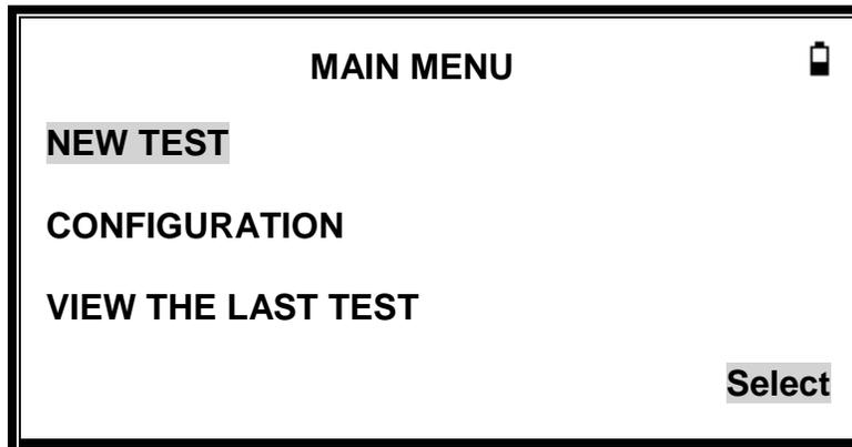
A battery state indicator
