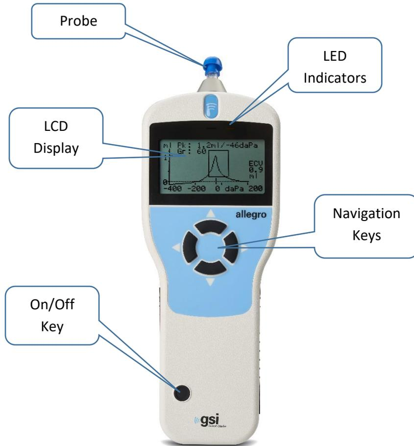
Press the On/Off key momentarily to turn the GSI Allegro on (refer to the diagram above). No warm-up time is required, although a short diagnostic routine will run for a few seconds. During this time the internal pump will operate. To switch off, again press and hold the On/Off key for a few seconds.
