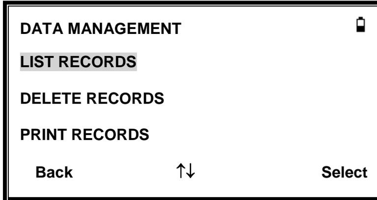
LIST RECORDS is used to work with the record of an individual test. All other options operate on groups of records.
