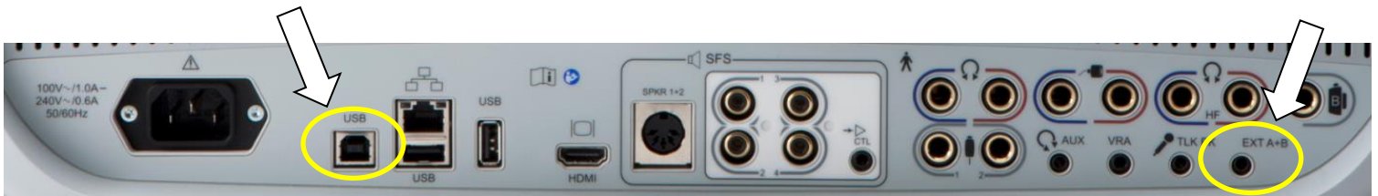
AudioStar Pro rear panel – USB and External Input ports
