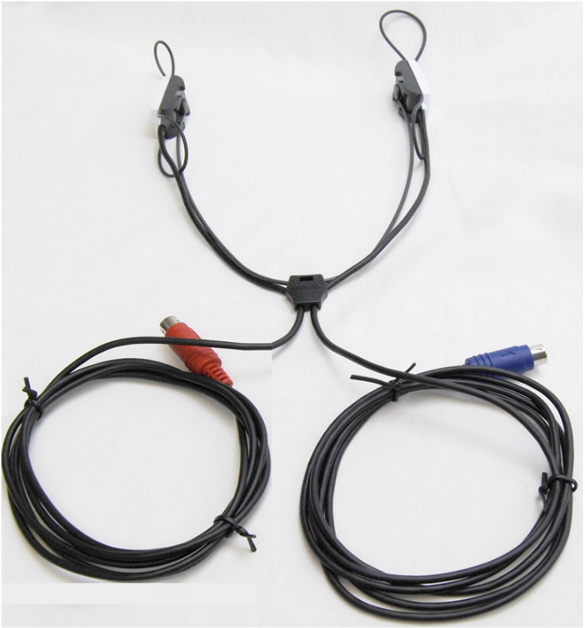
Probe Mic Hanger installation assembly complete.
