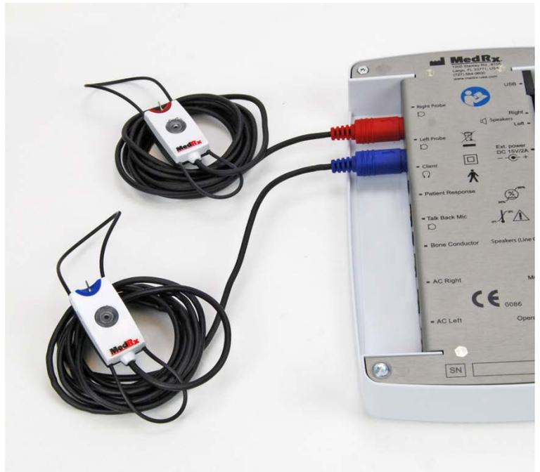
Connect the probe microphones to the AVANT ARC main unit. DO NOT force the connector into the jacks. Align correctly before insertion.
