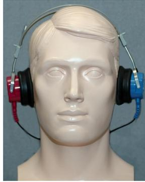
1. Place the earphones on the patient's head so the center of the earphone is directly over the opening of the ear canal.
