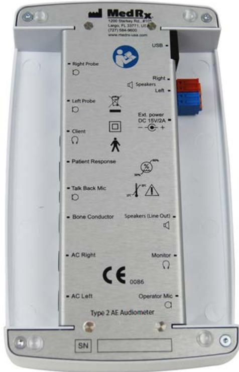
Connect the peripherals before testing a patient. Using the pictures below, locate each of the accessories and plug them into the unit.
