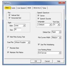
The **View** tab allows you to set the default appearance of the REM test environment. Defaults can be changed by using the check boxes and pull-down menus shown above.
