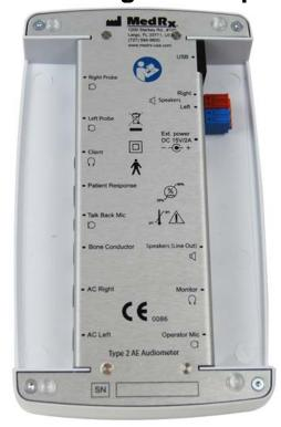
Connect the peripherals before testing a patient. Using the pictures below, locate each of the accessories and plug them into the unit.
