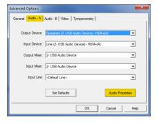
Use the **Audio-A** Tab to select the proper audio device for your Avant ARC. This tab also provides access to the **Windows Audio controls**.
