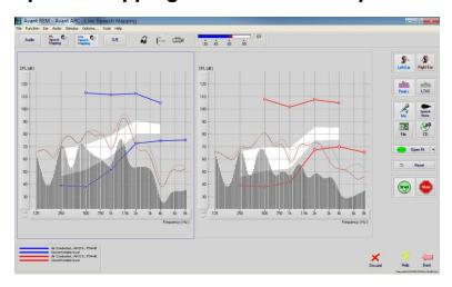
The screenshot on the left shows the Live Speech Mapping (LSM) window. The system is designed to capture and display the human voice in the ear canal, so it is recommend to use the microphone input and the peaks measurement.
