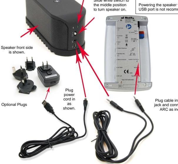
Plug cable into speaker jack and connect to your ARC as indicated.
