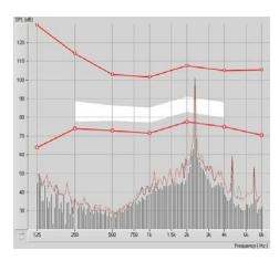
If a more specific frequency analysis of the feedback is desired, change the resolution of the system to 1/24 octave by clicking the **Options** menu item and changing the Analyzer selection using the pull-down menu. This image shows the same feedback as above at **1/24** octave.
