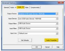
Use the **Audio-B** Tab to select the proper audio device for your AVANT ARC. This tab also provides access to the **Windows Audio controls**.
