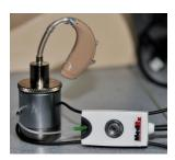
Note: If the REAR and the coupler response were measured with the insert headphone, the program saves the coupler response curve for later use. In this case to obtain another RECD, only REAR with insert headphone measurement is necessary. This is possible because the coupler response does not change provided that *neither the coupler nor the insert earphone has changed*.
