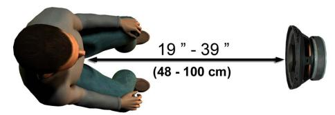
Make sure the grill of the loudspeaker is level with and directly in front of the patient's head.
