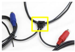
Turn clip over place probe mic wires into clip
