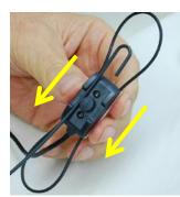
Install the hook on the back side of probe mic
