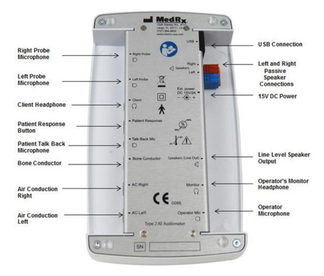
**Notice!** The Red & Blue adapters are included and must be removed to attach 18 gage (1.0mm) Free Field speaker wires and then reinstalled. DC Power supply must be used when using passive Free Field speakers.
