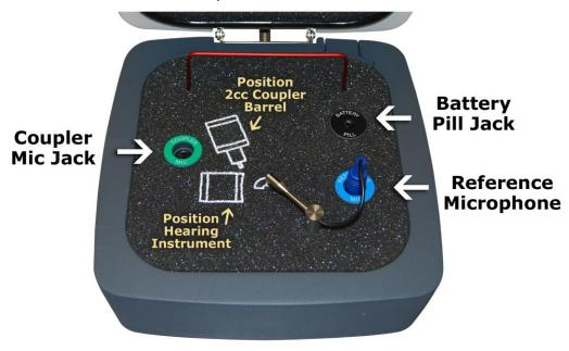
Inside the Test Chamber
