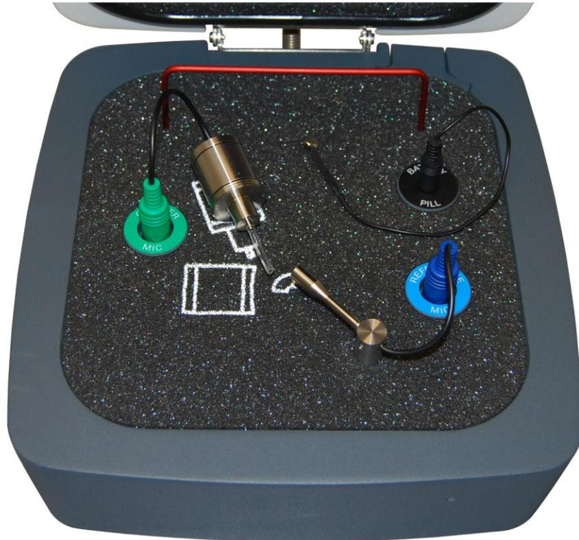
Carefully install the coupler microphone (green) as shown in the image above. Take care when handling these components, as they are delicate, precision calibrated instruments.
