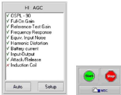
Click **Start** to start a single test in automatic mode. The test will finish after the measurement is complete.
