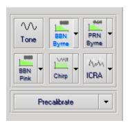
The signal type can be selected from this toolbar. The noise signal buttons can be re-assigned with desired noise types and weights from drop down lists. These assignments will be stored for quick signal selection.
