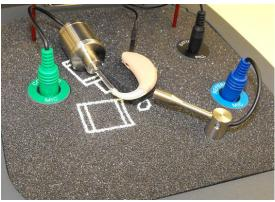
Place the aid on a foam pad or other material if needed to raise the sound inlet to the level of the reference microphone, with a 2-8mm separation distance.
