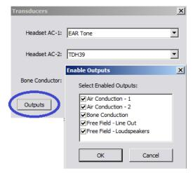
To add or remove outputs, click **Outputs** to enable or disable transducer buttons on the Audiometry screen
