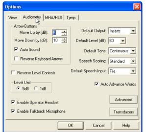
The Audiometry tab sets the look and behavior of the AVANT Stealth Audiometer.
