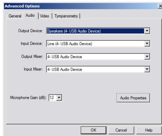
Use the Audio Tab to select the proper audio device for your AVANT Stealth Audiometer. This tab also provides access to the Windows Audio controls. Note: The device settings may vary with different computers. Consult technical support before changing.
