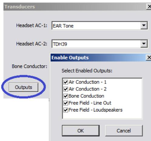
To add or remove outputs, click **Outputs** to enable or disable transducer buttons on the Audiometry screen
