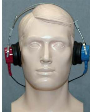
1. Place the earphones on the patient's head so the center of the earphone is directly over the opening of the ear canal.
