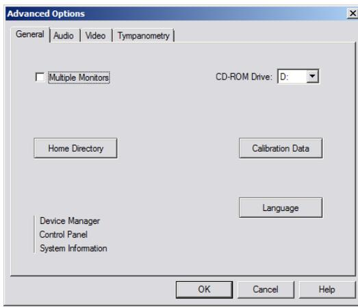
The General Tab configures the overall AVANT Stealth Audiometer behavior with respect to other Windows programs, specifically NOAH.
