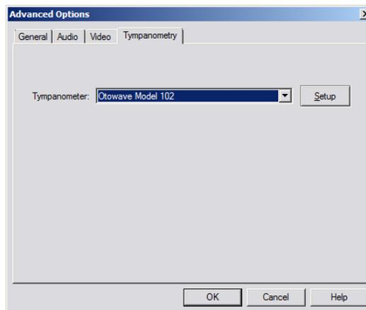
If your system has a Tympanometer connected, use this tab to identify it and ensure the driver and software that control it are correctly installed.
