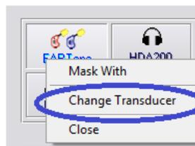
The Transducers dialog box will then appear. Select the appropriate transducer for each output.
