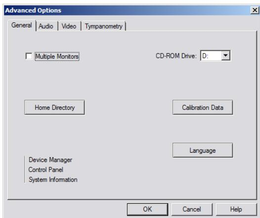
The General Tab configures the overall AVANT Stealth Audiometer behavior with respect to other Windows programs, specifically NOAH.
