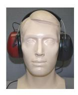
Place the earphones on the patient's head so the center of the earphone is directly over the opening of the ear canal.
