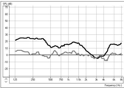
The top curve indicates significant occlusion effect. The lower curve is a close match to the normalized zero line and does not indicate significant occlusion effect.
