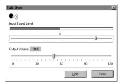
Speak at a normal level and calibrate the Input Sound Level to the microphone by sliding the arrow icon until the blue line on the VU meter just meets the calibration marker. When you see the VU meter line go past this marker, the line will be red. In this case, you have adjusted it too high.
