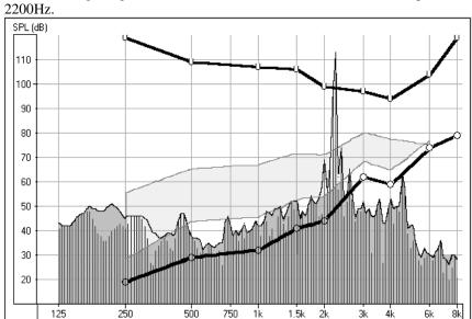
The following diagram illustrates feedback with a fundamental peak frequency at 2200Hz.
