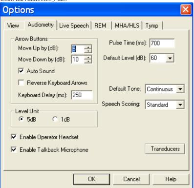
Features you can customize include: arrow icons (step size); Autosound; reverse keyboard arrows; Keyboard delay time; pulse time; default level; talkback level; enable operator headset and talkback microphone; Level increments; speech scoring (UK); default Tone and control of multimedia speakers.
