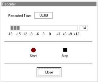
The talkover microphone is activated, although there is no output to the speakers as yet. Have the third party member practice speaking the intended speech sample into the microphone. Aim to peak the voice effort at zero on the active VU meter.
