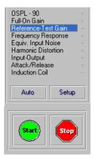
Adjust the hearing instrument volume control to the meet the reference test gain required.
