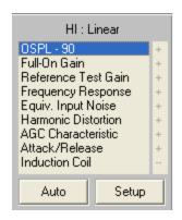
The test setup screen displays a list of Unselected and Selected tests. To move a test from one column to another, click on the test description and then the *arrow* icon pointing in the direction you want to move the test to.
