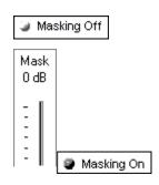
When masking is required, click *Masking Off* to turn the masking narrow band noise on. The icon will now indicate Masking ON. Masking noise automatically routes to the non-test ear. Therefore, if you are testing right bone conduction and you select Masking, the masking noise automatically routes to the left insert earphone. Remember to place the air conduction insert earphone in the non-test ear for masking.
