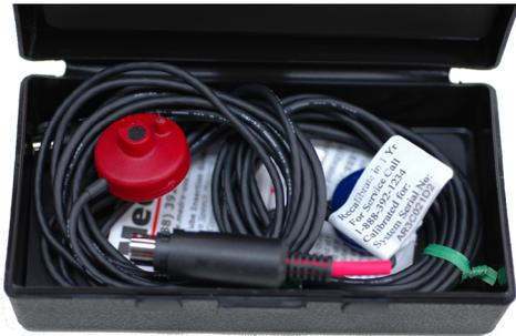
2. Carefully remove the probe microphones. Note that these are precision instruments and must be handled with care. Avoid dropping them or striking them against hard surfaces such as counter or desktops.
