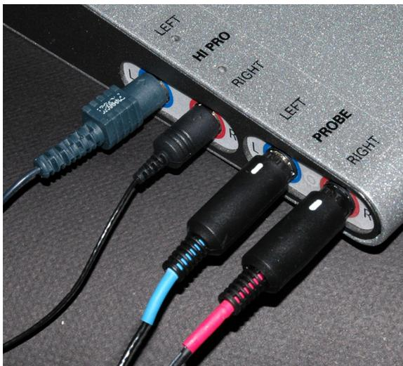
1. Locate the appropriate Hi-PRO cable as instructed by the Hearing Instrument Manufacturer.
