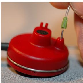
2. Place the probe tube between the calibration nibs as shown. Be sure that the opening of the probe tube is centered on the grill of the reference microphone.
