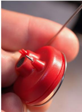
1. Hold the probe microphone assembly so that with the ear hook is facing the front of the head, the microphone ports face away from the patient.
