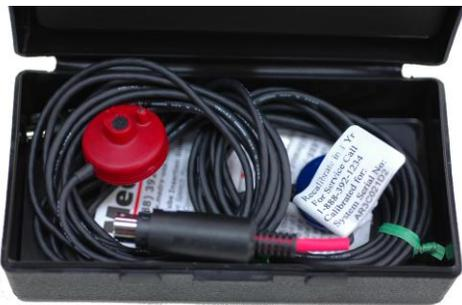
2. Carefully remove the probe microphones. Note that these are precision instruments and must be handled with care. Avoid dropping them or striking them against hard surfaces such as counter or desktops.
