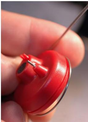
1. Hold the probe microphone assembly so that with the ear hook is facing the front of the head, the microphone ports face away from the patient.
