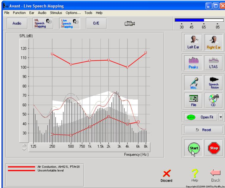
The screenshot on the left shows the Live Speech Mapping (LSM) window. The system was designed to capture and display the human voice in the ear canal, so we recommend using the microphone input and peak measurement.
