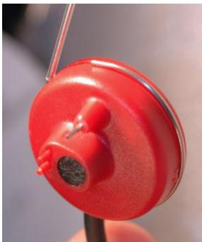
3. Carefully snap the wire loop into the groove and rotate the probe microphone assembly so the ear hook is on top and the black microphone cable is on the bottom.
