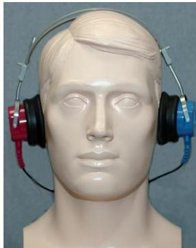
1. Place the earphone on the patient's head so the center of the earphones is directly over the opening of the ear canal.
