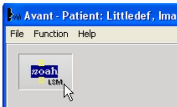
2. From the AVANT™ main screen, click the NOAH LSM button. The AVANT™ LSM window will reduce in size and "float" on top of the NOAH screen.
