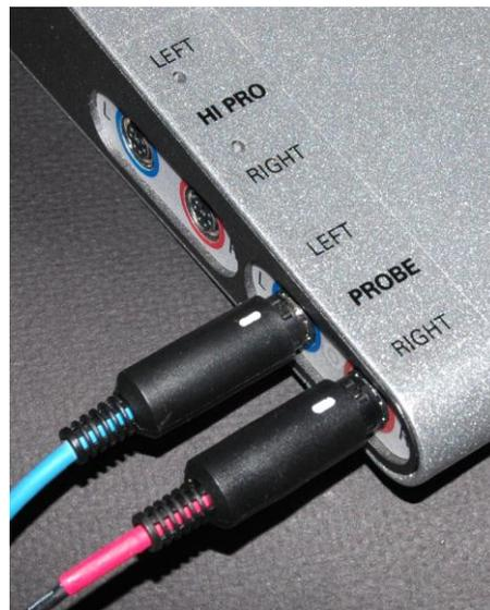
3. Connect the probe microphones to the AVANT™ main unit as shown above. The cables will only connect when the white mark on the cable connector faces straight up.
