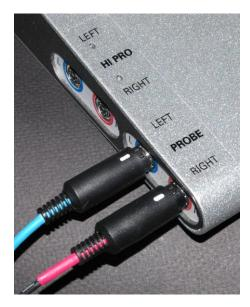
3. Connect the probe microphones to the AVANT<sup>™</sup> main unit as shown above. The cables will only connect when the white mark on the cable connector faces straight up. **DO NOT FORCE THE CONNECTOR INTO THE SOCKET.**
