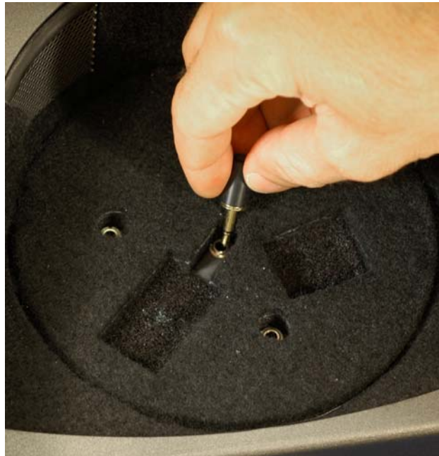
Install the Reference Microphone as shown above.
