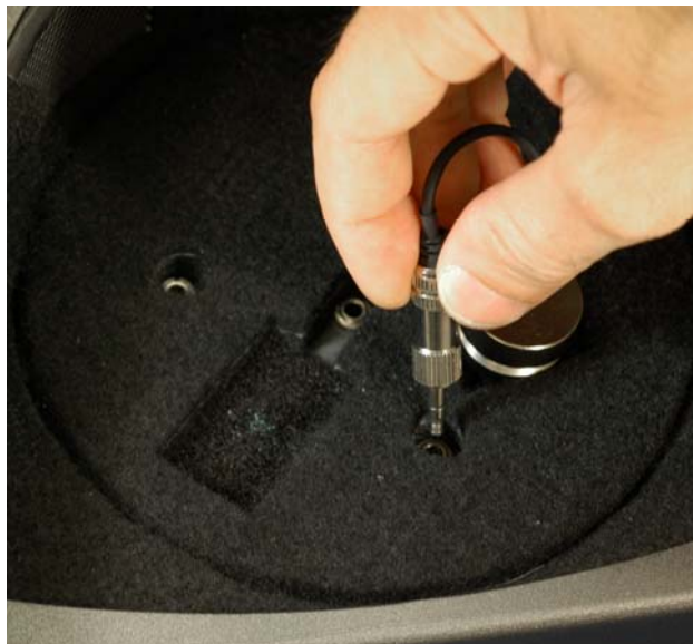
Install the Coupler Microphone as shown above.
