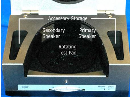
Inside the Test Chamber
