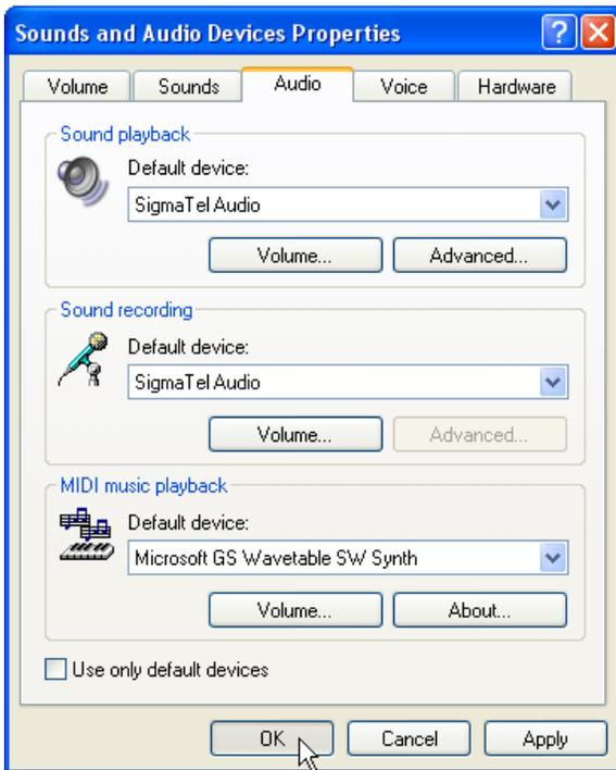
5. Using the pull downs, set the Sound Playback and Sound Recording Default devices to the internal sound card of your computer.
