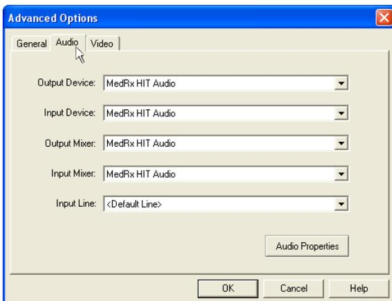
7. When the audio properties are configured properly, the Audio Tab will appear like the image on the left. If not, use the pull-down lists to adjust the settings to match the image.
