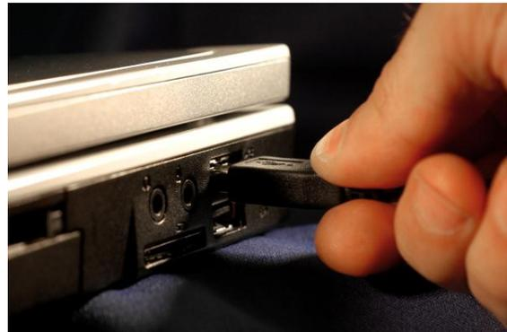
1. Connect the USB cable from the AVANT POLAR HIT™ to your computer as shown above.
