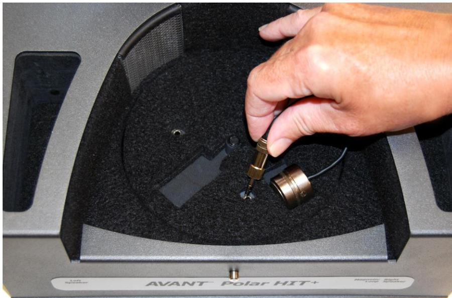
Install the Coupler Microphone as shown above.
