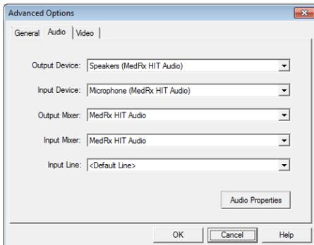
4. When the audio properties are configured properly, during driver installation, the Audio Tab will appear like the image on the left. If not, use the pull-down lists to adjust the settings to match the image.
