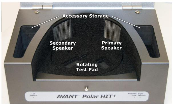
Inside the Test Chamber
