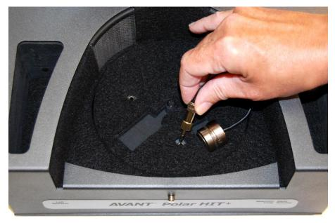
Install the Coupler Microphone as shown above.
