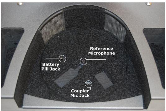
Detail view of the Rotating Test Pad
