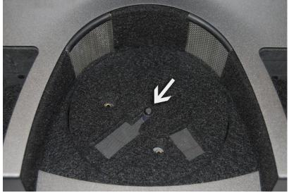
Carefully install the coupler microphone as shown in the images below. Take care when handling these components, as they are delicate, precision calibrated instruments.
