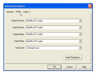
When the audio properties are configured properly, the Audio Tab will appear like the image on the left. If not, use the pull-down lists to adjust the settings to match the image.
