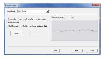
The calibration date is available under the **Function > Calibrate > Calibration** Information tabs. Return Probe Microphones to MedRx for annual re-calibration. Annual re-calibration of the Avant REM+ Probe Microphones is recommended. There are no user repairable components of this device.
