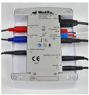
Headphones for use with REM devices should have 32 ohms impedance and the speaker power should be at least 5 watts.
