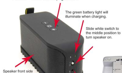
The front side of the speaker is placed at a distance of about 1 meter (19"-39") from the patient, for normal use.
