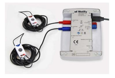
2. Connect the probe microphones to the AVANT REM+ main unit. DO NOT force the connector into the jacks. Align correctly before insertion. A cable from the "Speaker" jack on the REM+ will connect to the input jack in the powered speaker supplied with your unit.
