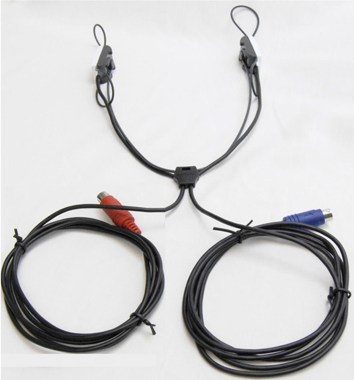
Probe Mic Hanger installation assembly complete.
