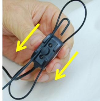
Install the hook on the back side of probe mic
