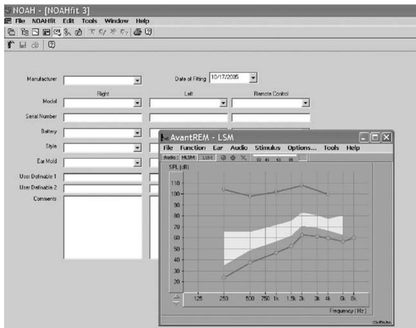
**You are now ready to make programming changes to the hearing instrument from the fitting software, while simultaneously monitoring the outcome on the REM LSM display.**
