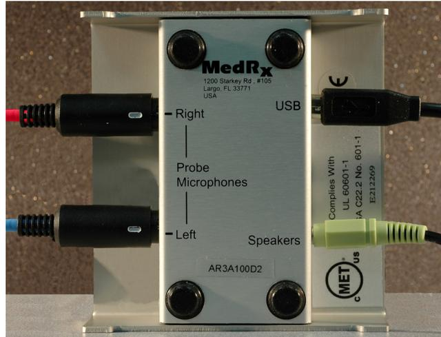
3. Connect the probe microphones to the AVANT REM Speech main unit as shown above. The cables will only connect when the white mark on the cable connector aligns with the black mark on the main unit. DO NOT force the connector on.
