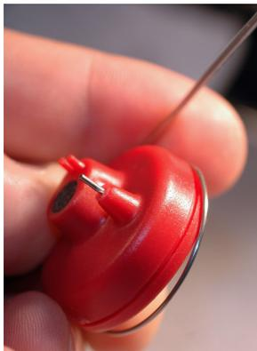
1. Hold the probe microphone assembly so that with the ear hook facing the front of the head, the microphone ports face away from the patient.
