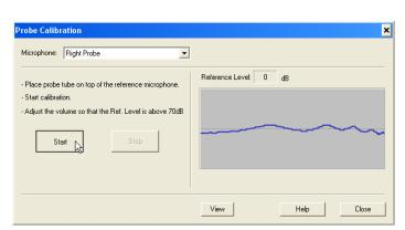
The calibration date is available under the Function > Calibrate > Calibration Information tabs. Return Probe Microphones to Medrx for annual re-calibration.
