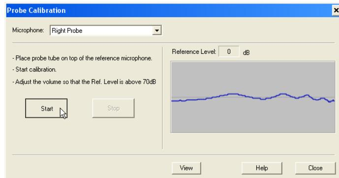
Repeat for the other probe. Valid calibrations have the same approximate shape as the gray target curve. If the measured calibration curve differs greatly in shape or amplitude from the gray target curve, replace the probe tube and re-calibrate. If this does not correct the problem, contact MedRx technical support at (888) 392-1234.
