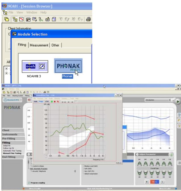
Open the fitting module from the NOAH Module Selection Screen.
