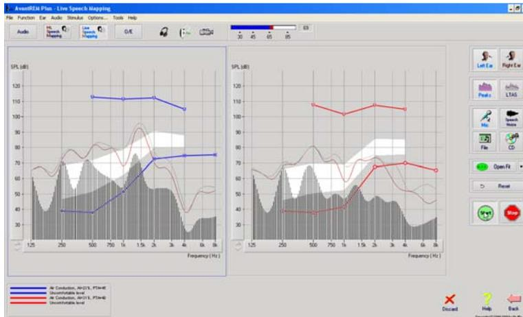
The screenshot on the left shows the Live Speech Mapping (LSM) window. The system was designed to capture and display the human voice in the ear canal, so we recommend using the microphone input and the peaks measurement.
