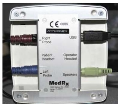
2. Connect the probe microphones to the AVANT REM Speech<sup>+</sup> main unit as shown above. **DO NOT** force the connector on.
