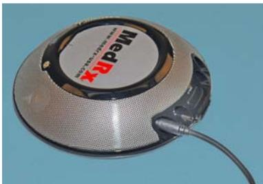
1. Plug speaker wire in. The speaker may be battery powered or plugged into the plug-in power supply that is included.
