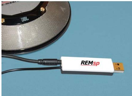
2. Connect the speaker to the AVANT REMsp main unit as shown above. DO NOT force the connector on. Turn on the speaker and hold down the (+) button to set the maximum volume.
