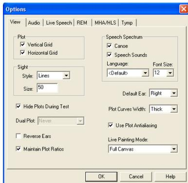
The **View** tab allows you to set the default appearance of the REMsp test environment. Values can be changed by using the check boxes and pull-down menus shown above.
