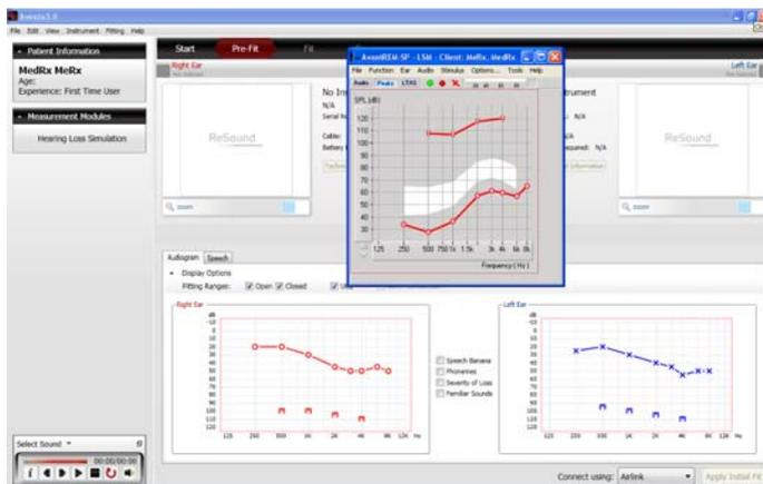
Use the text menus and green and red buttons in the floating LSM window to make Speech Mapping measurements. Make necessary changes to the instrument based on these measurements. To make adjustments to the hearing instrument, click on the fitting module window and modify the settings according to the manufacturer’s instructions, being sure to activate, apply or save the settings to the instrument.
