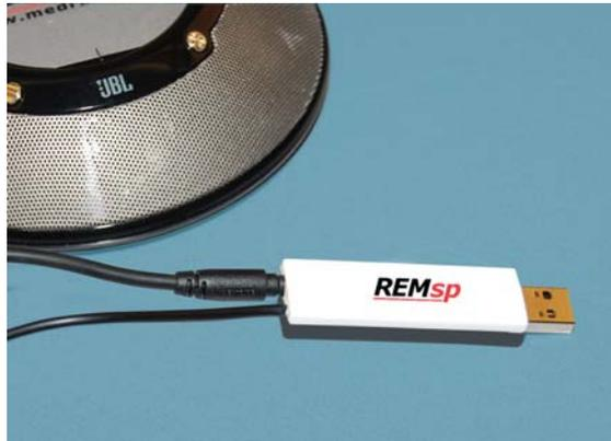
2. Connect the speaker to the AVANT REMsp main unit as shown above. DO NOT force the connector on. Turn on the speaker and hold down the (+) button to set the maximum volume.
