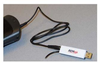
2. Connect the speaker to the AVANT REMsp main unit as shown above. Turn on the speaker and hold down the (+) button to set the maximum volume.
