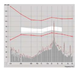
If a more specific frequency analysis of the feedback is desired, change the resolution of the system to 1/24 octave by clicking the **Options** menu item and changing the Analyzer selection using the pull-down menu. This image shows the same feedback as above at 1/24 octave.
