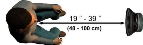
Make sure the grill of the loudspeaker is level with and directly in front of the patient's head.
