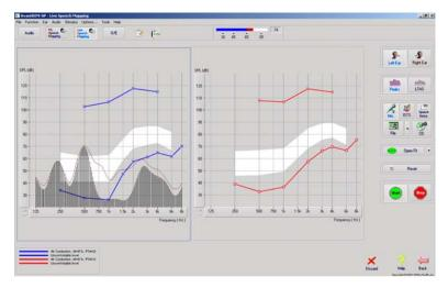
The screenshot on the left shows the Live Speech Mapping (LSM) window. The system was designed to capture and display the human voice in the ear canal, so we recommend using the microphone input and the peaks measurement.
