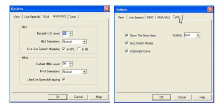
The **MHA/ HLS** tab sets the default look and behavior of the Master Hearing Aid and Hearing Loss Simulator. If your system has a **Tympanometer** connected, this tab will assist in configuring the look of the display.
