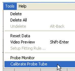
Position probe microphone between 19 and 39 inches from the loudspeaker and click Start. The signal must be at least 70 dB to complete a valid calibration. If the screen prompt indicates the signal is too low, increase the volume on the loudspeaker or move the probe microphone assembly closer and restart the calibration.
