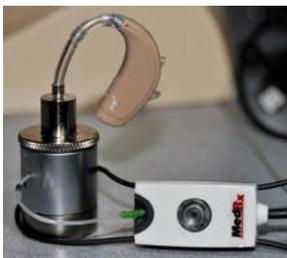
Note: If the REAR and the coupler response were measured with the insert headphone, the program saves the coupler response curve for later use. In this case to obtain another RECD, only Ear Response with insert headphone measurement is necessary. This is possible because the coupler response does not change provided that *neither the coupler nor the insert earphone has changed*.
