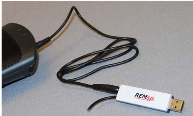
2. Connect the speaker to the AVANT REMsp main unit as shown above. Turn on the speaker and hold down the (+) button to set the maximum volume.
