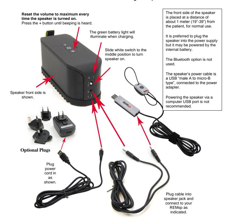
**Speaker Calibration:** open the Speaker Calibration screen from REM/LSM screen menu **Tools**>**Calibrate Speakers**.
