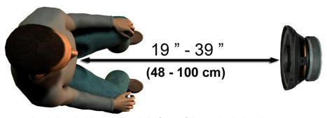
Make sure the grill of the loudspeaker is level with and directly in front of the patient's head.
