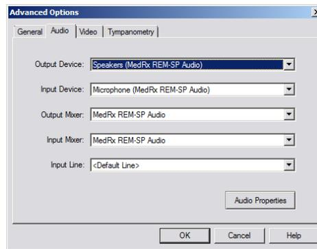
Use the **Audio Tab** to select the proper audio device for your Avant REMsp. This tab also provides access to the Windows Audio controls.
