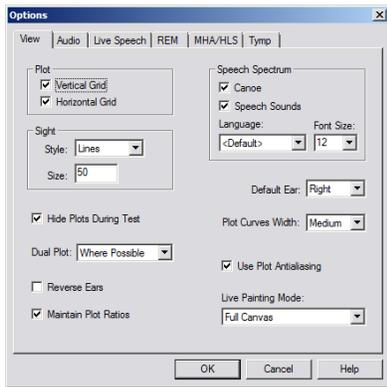
The **View** tab allows you to set the default appearance of the REMsp test environment. Values can be changed by using the check boxes and pull-down menus shown above.
