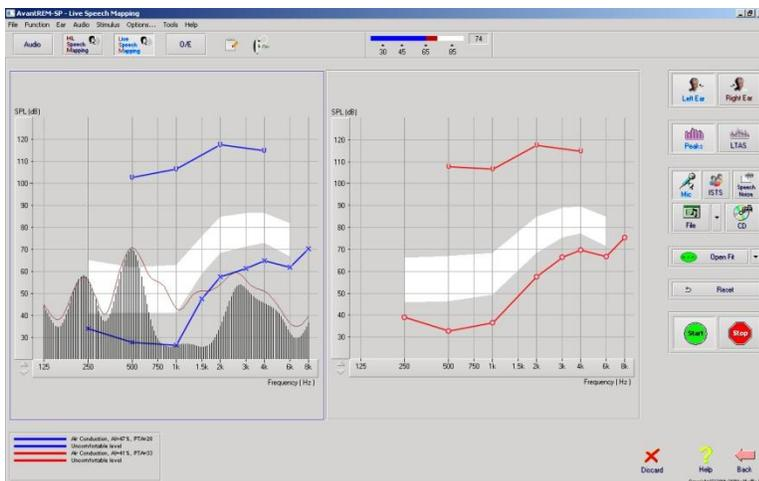
The screenshot on the left shows the Live Speech Mapping (LSM) window. The system was designed to capture and display the human voice in the ear canal, so we recommend using the microphone input and the peaks measurement.
