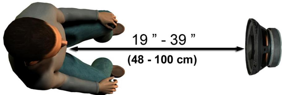
Make sure the grill of the loudspeaker is level with and directly in front of the patient's head.
