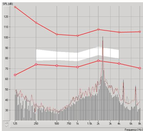
If a more specific frequency analysis of the feedback is desired, change the resolution of the system to 1/24 octave by clicking the **Options** menu item and changing the Analyzer selection using the pull-down menu. This image shows the same feedback as above at **1/24 octave**.
