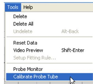
Position probe microphone between 19 and 39 inches from the loudspeaker and click **Start**. The signal must be at least 70 dB to complete a valid calibration. If the screen prompt indicates the signal is too low, increase the volume on the loudspeaker or move the probe microphone assembly closer and restart the calibration.
