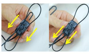
Install the hook on the back side of probe mic
