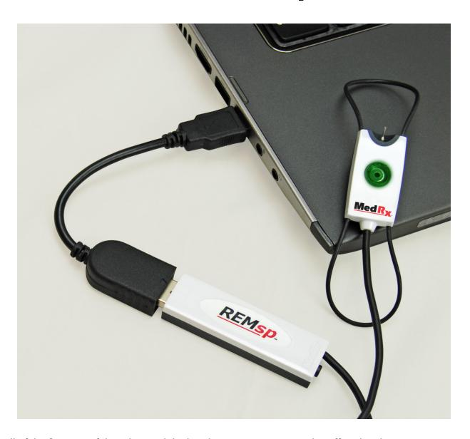
All of the features of the advanced dual probe AVANT REM+ are also offered in the AVANT REMsp. (See the AVANT REM+ for features) The REMsp is a single probe comprehensive REAL EAR Measurement and Live Speech Mapping system that is remarkably small. Measuring only about 3.25 inches long, this device plugs into the USB port of the computer.
