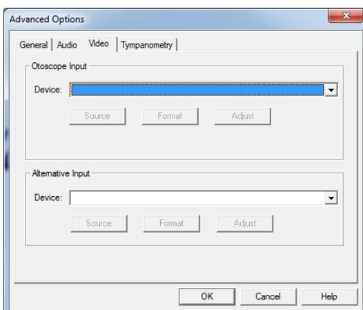
If your system has a Video Otoscope, the **Video** tab allows you to select the appropriate device driver.
