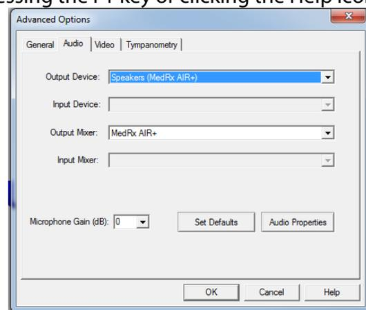
Use the **Audio** Tab to select the proper audio device for your Audiometer. This tab also provides access to the Windows Audio controls.
