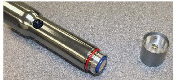
End cap removed showing battery in place. In normal use, the rechargeable battery will not need to be removed.
