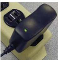
Green light on charger indicates a full charged battery when connected to the light handle.
