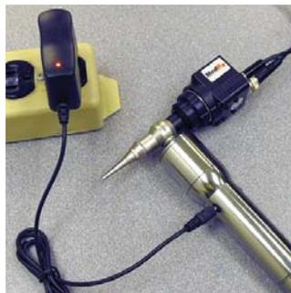
Connect charger to power outlet and plug small round connector into the hole on the side of light handle. (Note: light on top of the charger is orange when charging)
