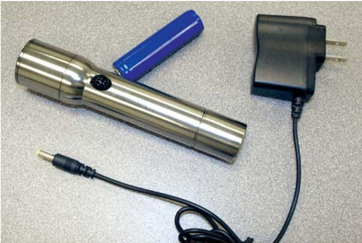
The LED light handle has three components: the Silver Light Handle, the Lithium-Ion battery (3.6 volt, rechargeable) and the Charger for the battery.
