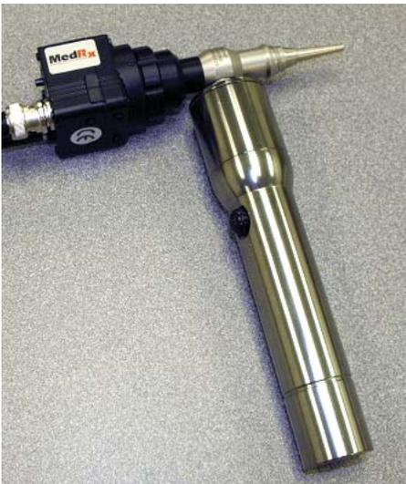
LED light handle installed on Otoscope. (Note: Black button to turn the light on and off)
