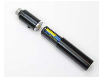
End cap removed showing batteries in holder and inserted into handle.
