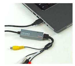
1. Connect the USB Capture Dongle to a USB port on your computer.
