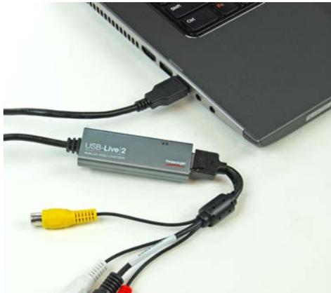
1. Connect the USB Capture Dongle to a USB port on your computer.
