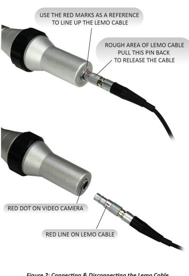
Figure 2: Connecting & Disconnecting the Lemo Cable
